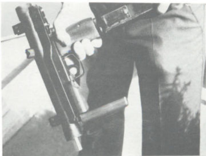
Inserting the magazine. Note the cocking handle locked in the rear position.
